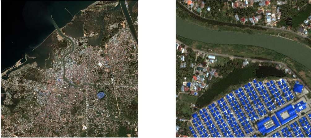
Figure 3: Left: The full pansharpened version of the tile seen in figure 2. Right: The pansharpened subset of the tile seen in figure 2. Note the combination of the spectral resolution of the multispectral image and the spatial resolution of the panchromatic image.
